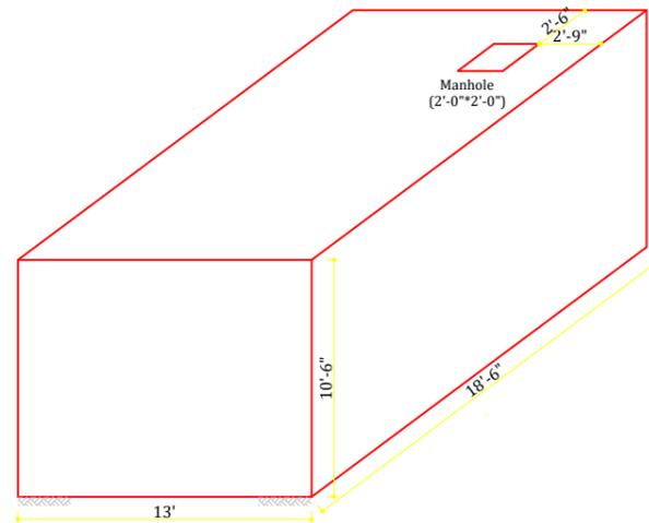
FIG.1: ISOMETRIC VIEW OF UNDERGROUND WATER TANK
